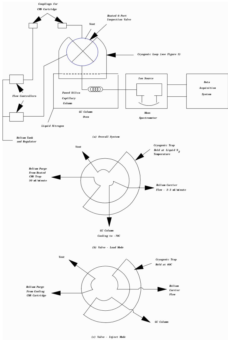
**FIGURE 3. GC/MS ANALYSIS SYSTEM FOR CMS CARTRIDGES**
