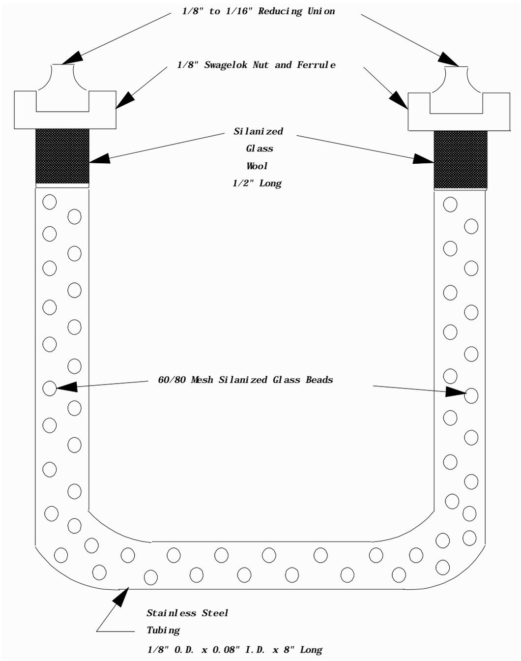
**FIGURE 5. CRYOGENIC TRAP DESIGN**
