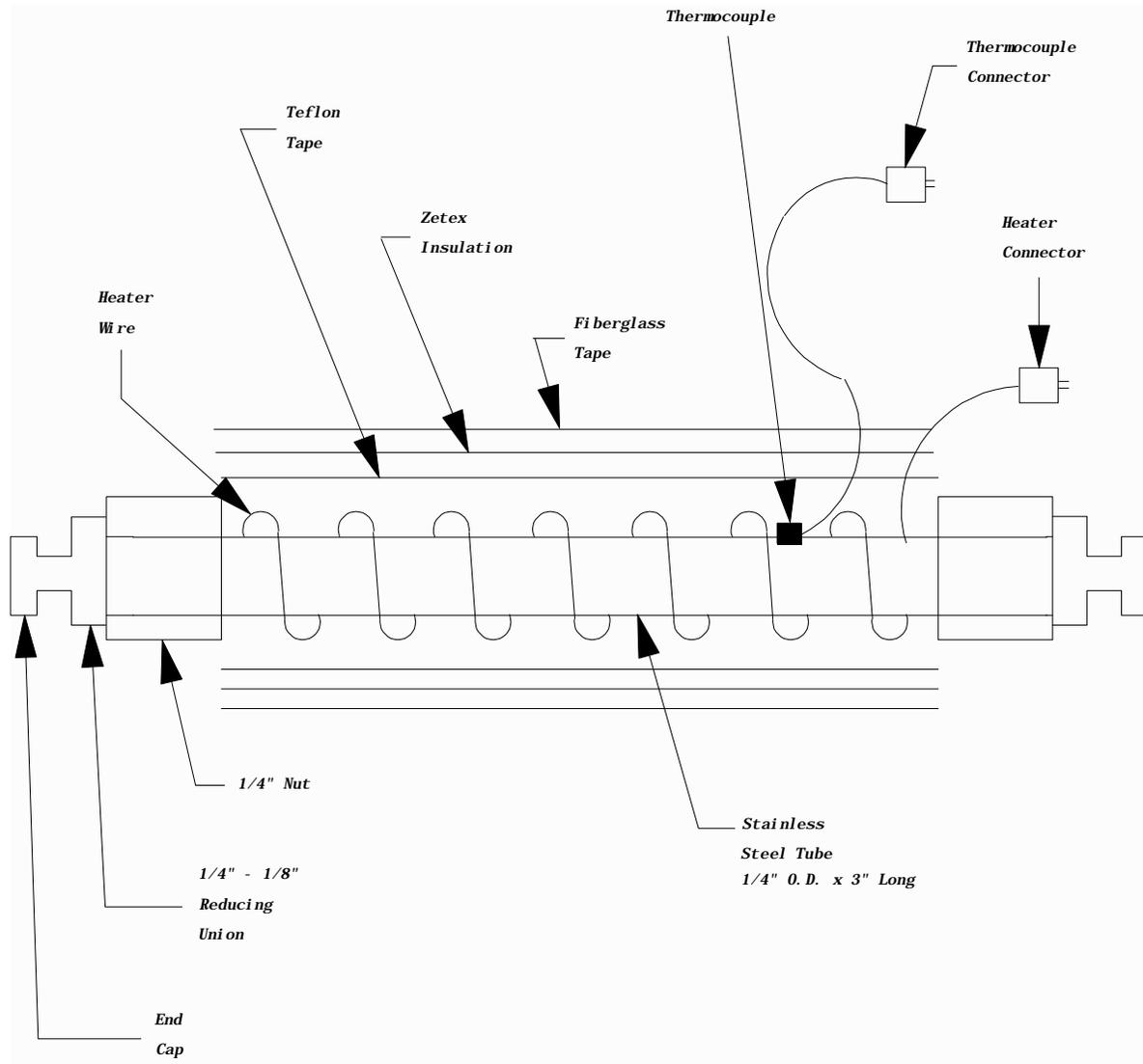
**FIGURE 1. DIAGRAM SHOWING CARBON MOLECULAR SIEVE TRAP (CMS) CONSTRUCTION**
