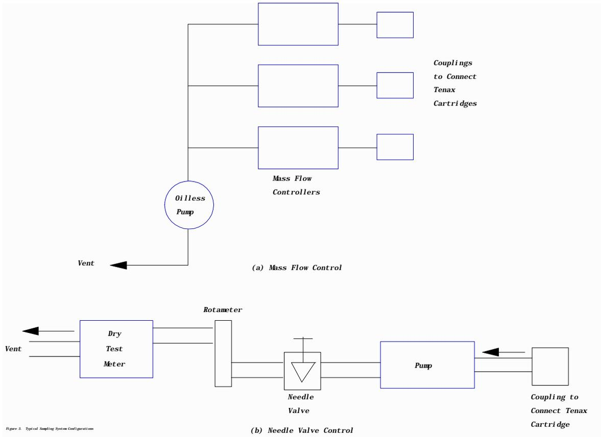
Figure 2. Typical Sampling System Configurations
